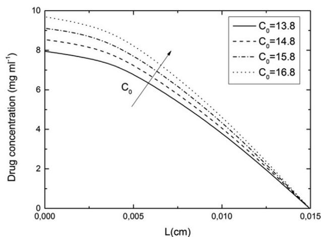
Fig. 4. Prediction of drug concentration inside the delivery device for  $t = 24$  h,  $L = 0.015$  cm,  $D = 5 \cdot 10^{-8}$  cm<sup>2</sup>/mn and for  $C_0 = 13.8$ ,  $14.8$ ,  $15.8$  and  $16.8$  mg/ml.
