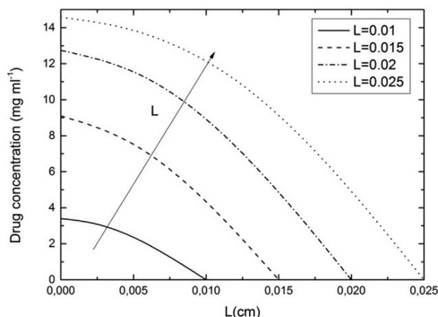
Fig. 5. Prediction of drug concentration inside the delivery device for  $t = 24$  h,  $D = 5 \cdot 10^{-8}$  cm<sup>2</sup>/mn and for  $C_0 = 15.8$  mg/ml and  $L = 0.01$ ,  $0.015$ ,  $0.02$  and  $0.025$  cm.
