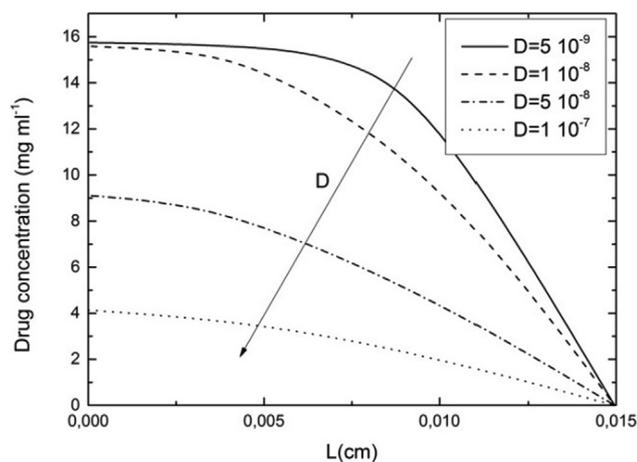
Fig. 3. Prediction of drug concentration inside the delivery device for  $t = 24$  h,  $L = 0.015$  cm,  $C_0 = 15.8$  mg/ml and for  $D = 5 \cdot 10^{-9}$ ,  $1 \cdot 10^{-9}$ ,  $5 \cdot 10^{-8}$  and  $1 \cdot 10^{-7}$  cm<sup>2</sup>/mn.
